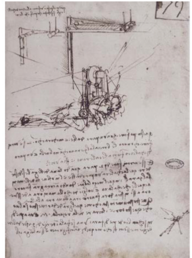
This detail of a flying machine shows a wing mechanism, which is being manipulated by a human pilot (sprawled out in the prone position).
